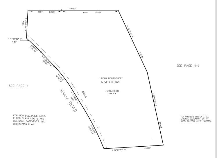
10' UTILITY & DRAINAGE EASEMENTS EACH SIDE OF PROPERTY LINES AS INDICATED BY DASHED LINES EXCEPT AS OTHERWISE SHOWN.
